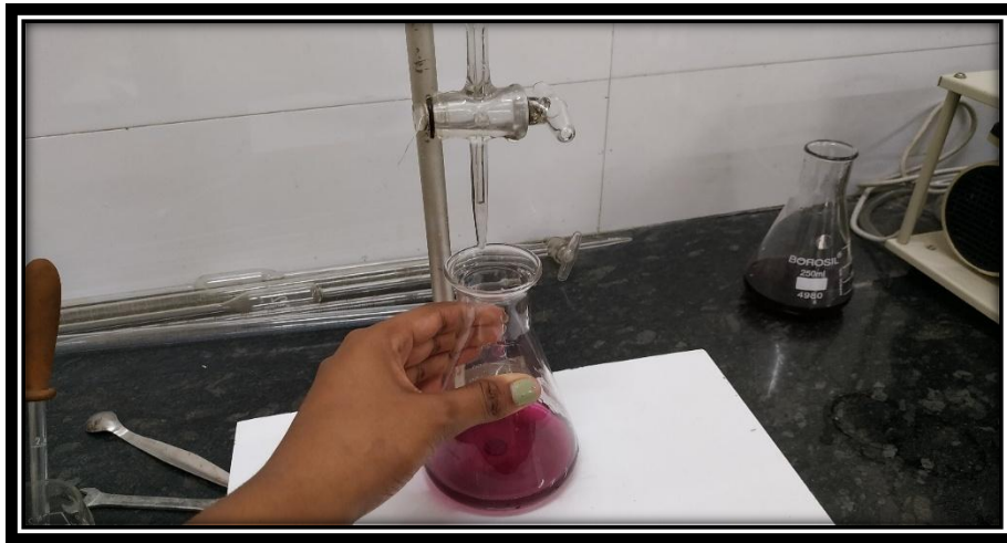
Figure 7. Determination of total hardness (by EDTA titrimetric method)
