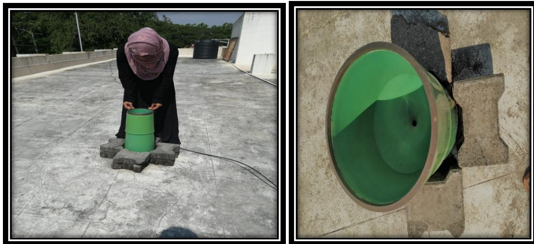
Figure 3. Rainfall Measurement from Ordinary Raingauge
